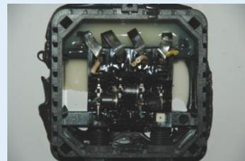
**Defect bypass diode**
