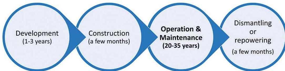
Figure 7: PV Plant Life Cycle
