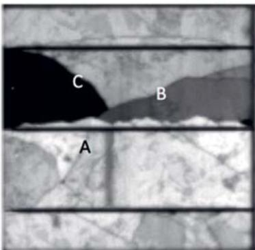
An adequate packing system of the PV modules that is able to withstand mechanical stress is key in order to transport the PV modules safely from the manufacturing to the installation site. Test revealed that no cell cracks occurred for vertical transport stacks while up to two Type A cracks per module were observed for the horizontal stacks. PV modules should hence be packed into vertical stacks to avoid damages during transport.
