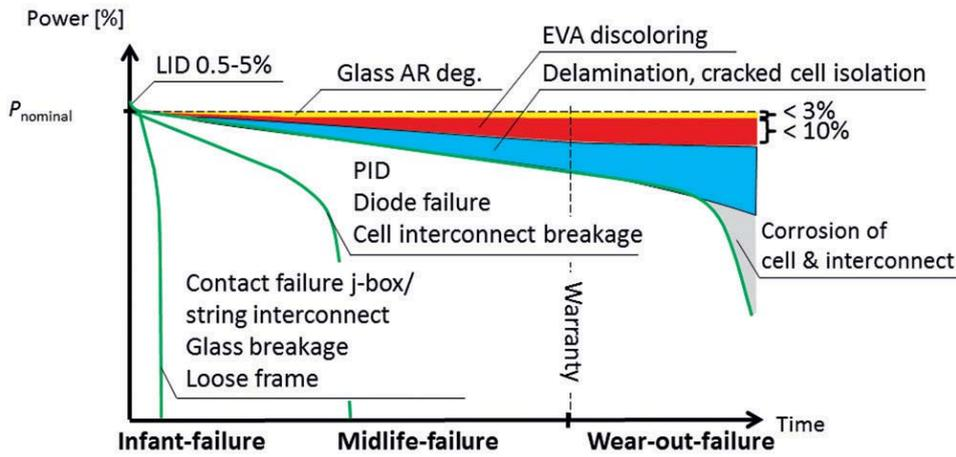
Figure 3: Typical failure scenarios for wafer based crystalline photovoltaic modules [29]
